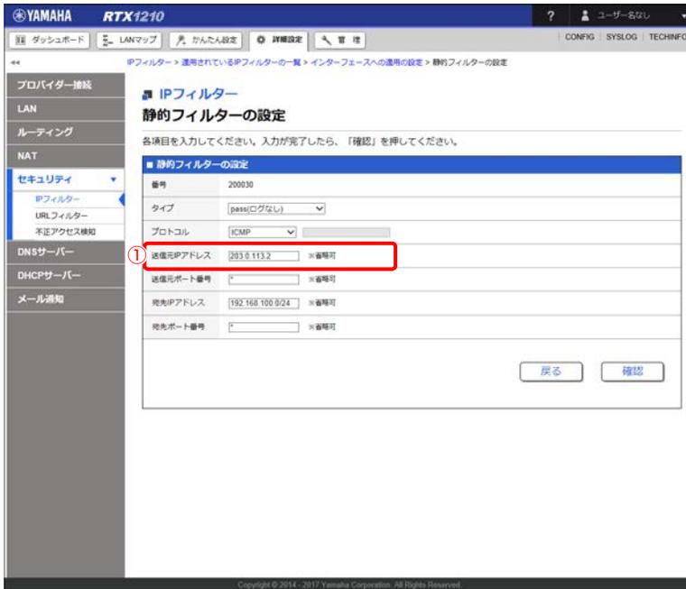
The screenshot shows the '静的フィルターの設定' (Static Filter Settings) page in the Yamaha RTX1210 web interface. The page title is '静的フィルターの設定' and it includes a sub-section '静的フィルターの設定'. The form contains the following fields:
